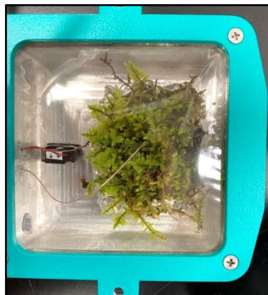
Figure 3. Hypnum imponens in the custom cuvette attached to the LI-6800
